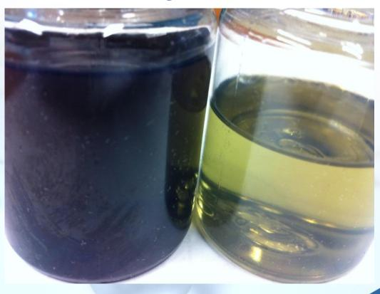
Fuel on left indicated high level of particulate Fuel on right shows level of cleanliness on single pass through Kleenoil Filter
